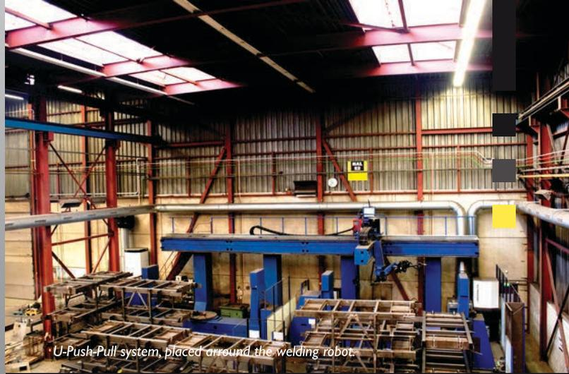
U-Push-Pull system, placed around the welding robot.
