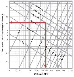
Example: for a 5 in. (125 mm) ST hose with airspeed of 4000 FPM (20 m/s), the static pressure loss w.g. per 100 feet is 11 in. and air volume is 350 CFM (10  $m^3/m$ ).
