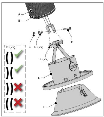
Fig. 4.3 Hood mounting (hose tube arm)
