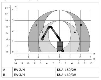
Fig. III Positioning of the extraction arm
