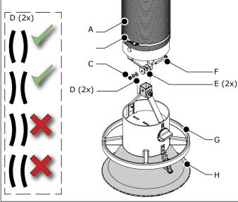
Fig. 4.4 Hood mounting (metal tube arm)
