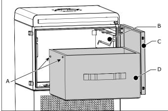
Fig. 6.2 Replacement of the HEPA filter cassette
