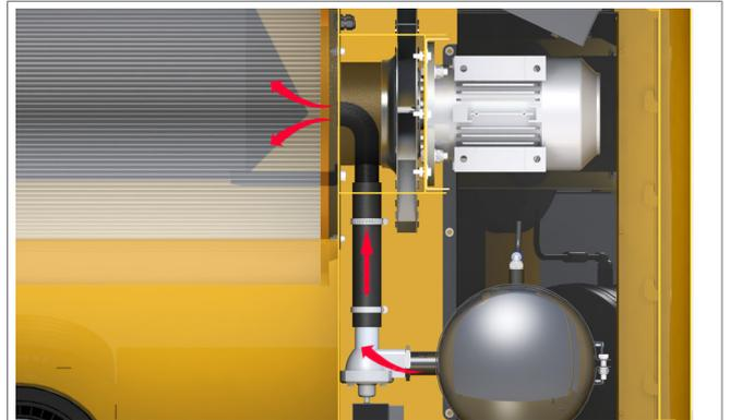
RamAir™ pulse amplifier: effective cleaning of the filter cartridge by powerful compressed air pulses
