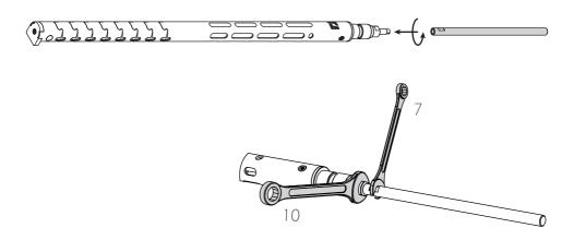
Thread the pull rod onto the snout and lock it in place.
