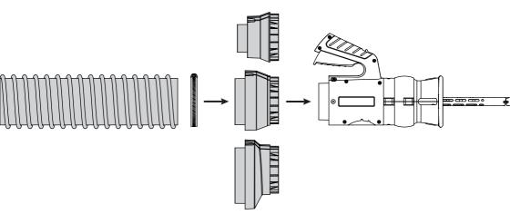
In case of a 75 mm / 3" hose, connect via the reducer. In case of a 125 mm / 5" or 150 mm / 6" hose, connect via an increaser.
