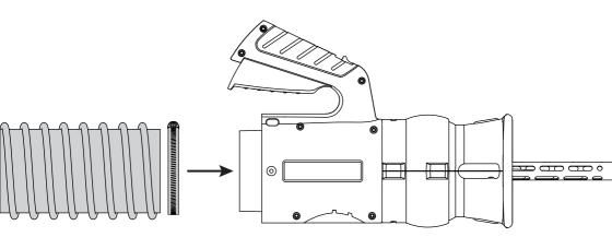
In case of a 100 mm / 4" hose, connect directly onto the grabber.
