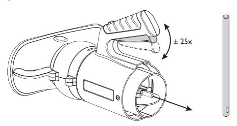
Continuously operate the handle until the pull rod can be removed from the rear.
