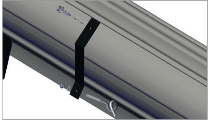
Fig. 5.3.8 Mounting the rope bracket
