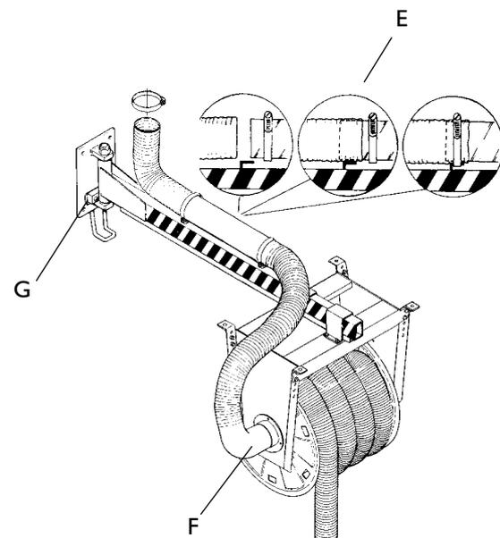
*Fig. 4.3.3d* Mounting duct to the boom arm
