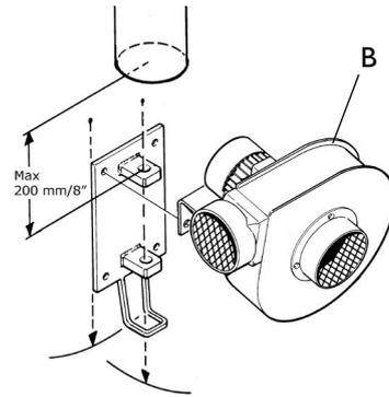
*Fig. 4.3.3b* Mounting the fan to the bracket
