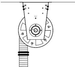
Fig. 4.2.2 Mounting hose reel on ceiling
