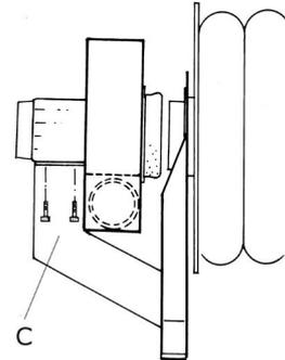
Fig. 4.3.1c Tightening the bolts on the DMF bracket
