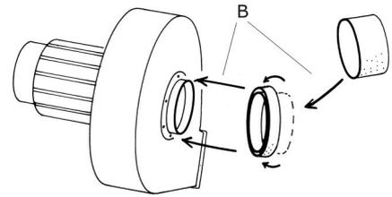
Fig. 4.3.1b Inserting the DMF bracket into the hose reel
