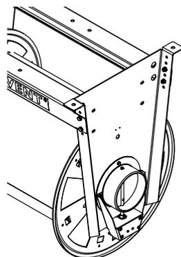
*Fig. 4.3.4* Mechanical damper
