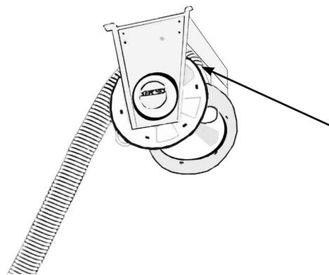
Fig. 4.2.2a Example of SER showing that at least a quarter turn of hose must remain on drum to prevent recoil mechanism from locking.
