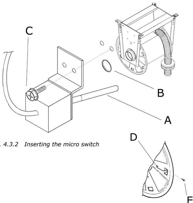
Fig. 4.3.2 Inserting the micro switch
