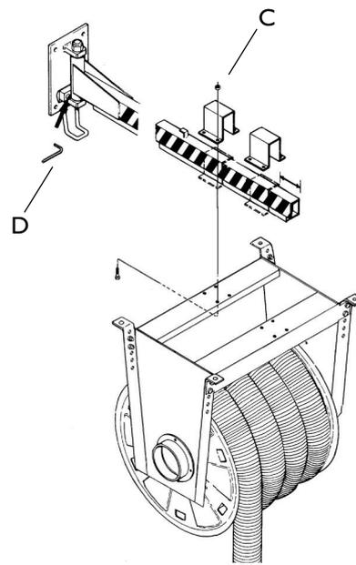
*Fig. 4.3.3c* Mounting the reel to the boom arm
