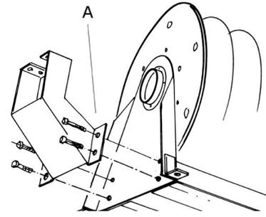
Fig. 4.3.1a Inserting the DMF bracket into the hose reel
