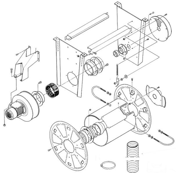
*Fig. 5.3* Replacing the plastic bearings
