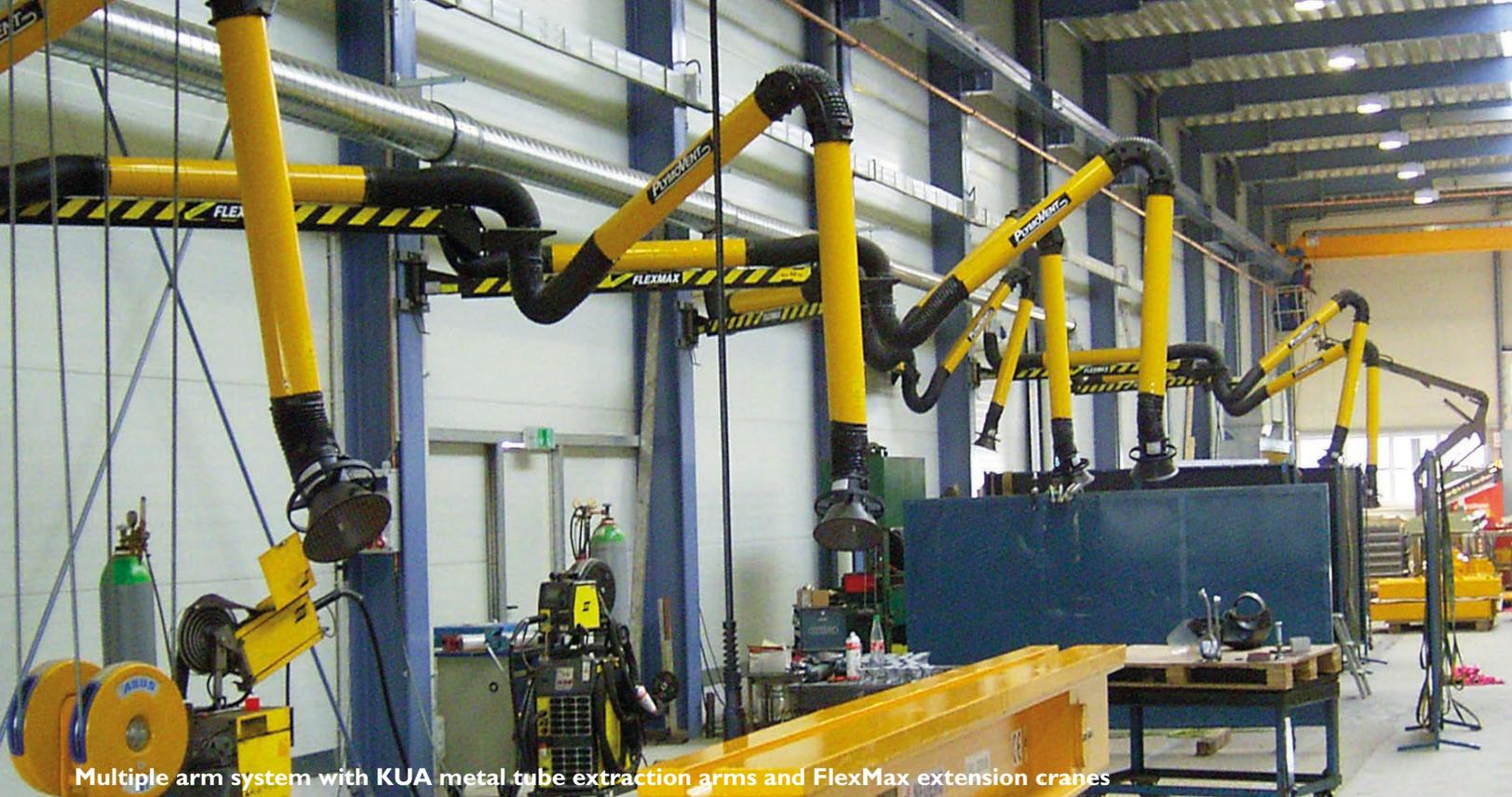
Multiple arm system with KUA metal tube extraction arms and FlexMax extension cranes
