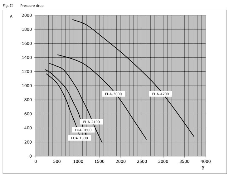
A = Static pressure (Pa) B = Airflow  $(m^3/h)$
