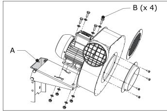
Fig. 4.2 Fan on mounting bracket MB-FUA/C1 or MB-FUA/C2
