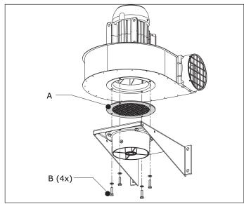
Fig. 4.4 Fan on arm bracket
