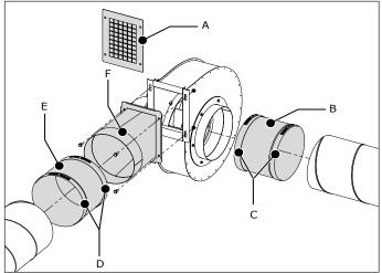
Fig. 4.6 Duct connection of the FUA-3000/4700
