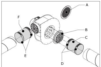
Fig. 4.5 Duct connection of the FUA-1800/2100
