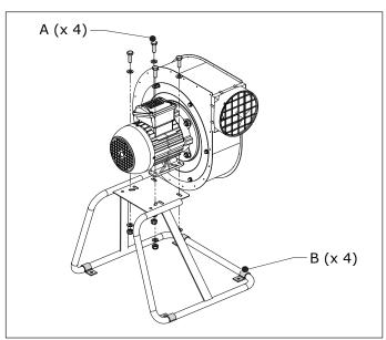
Fig. 4.1 Fan on mounting bracket MB-FUA/S1 or MB-FUA/S2
