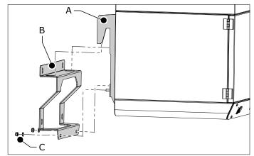
Fig. 4.1 Mounting of the wall bracket
