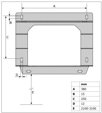
Fig. IV Positioning of the extraction arm
