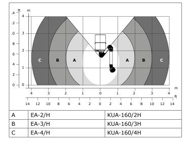
Fig. III Recommended installation height (E) + hole pattern
