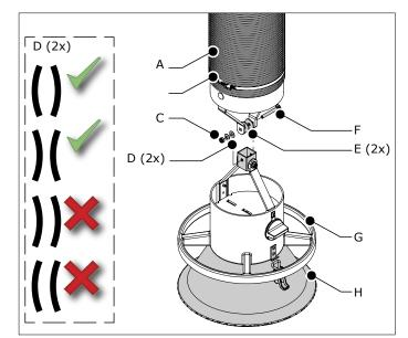
Fig. 4.4 Hood mounting (metal tube arm)
