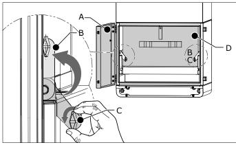
Fig. 6.2 Removal of the HEPA filter cassette
