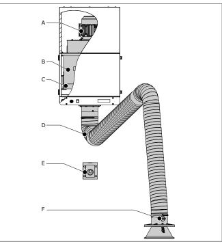
Fig. 2.1 Main components and elements
