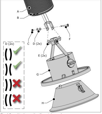
Fig. 4.3 Hood mounting (hose tube arm)
