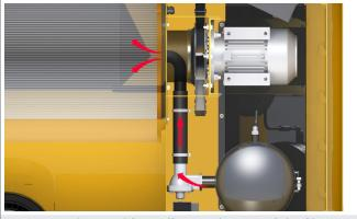
RamAir™ pulse amplifier: effective cleaning of the filter cartridge by powerful compressed air pulses
