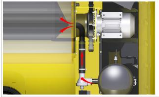
RamAir $^{\rm TM}$  pulse amplifier: effective cleaning of the filter cartridge by powerful compressed air pulses
