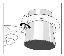
Position the Bayonet Quick Lock into the Magnetic Tailpipe Adapter and twist it clockwise until it stops.
