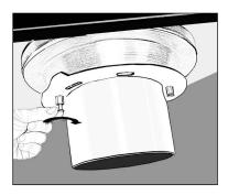
Twist the Bayonet Quick Lock counter clockwise and pull to remove from the Magnetic Grabber Tailpipe Adapter.
