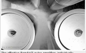
The effective RamAir™ pulse amplifier: individually cleaning of the filter cartridges by compressed air pulses
