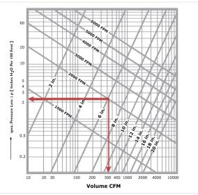
Example: for a 6 in. (150 mm) SNF2 hose with airspeed of 2000 FPM (10 m/s), the pressure drop per inch is 2.5 Pa and air volume is 300 CFM (8  $m^3/m$ ).
