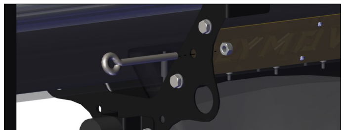
Fig. 6.3.4 Mounting the curl hooks on the crab.
