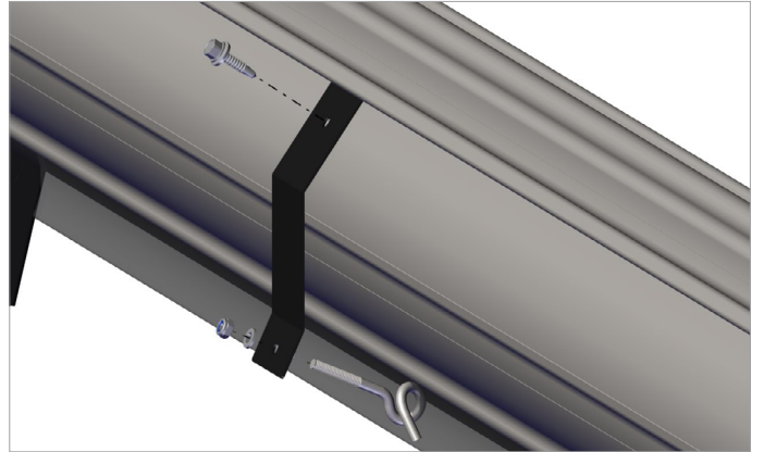
Fig. 5.3.8 Mounting the rope bracket
