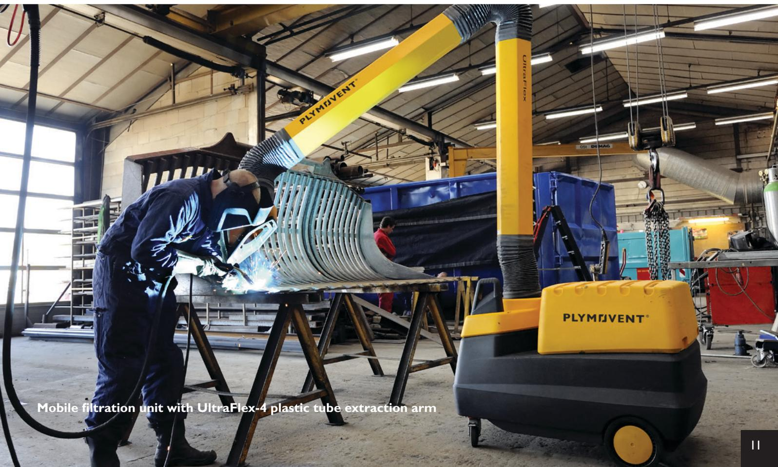
Mobile filtration unit with UltraFlex-4 plastic tube extraction arm
