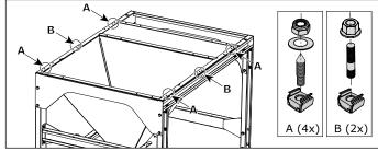
Fig. 4.15 Position of studs
