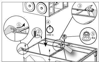
Fig. 4.14 Filter module on first frame
