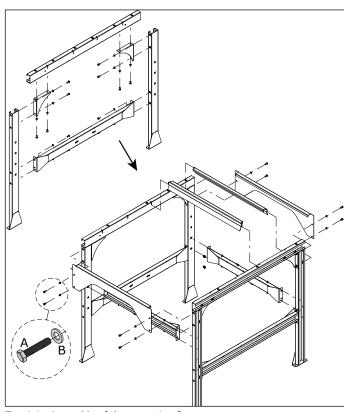
Fig. 4.1 Assembly of the mounting frame
