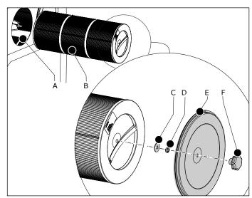
Fig. 4.27 Installation of the filter cartridges
