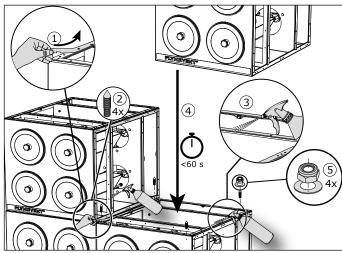
Fig. 4.20 Filter module on second filter module
