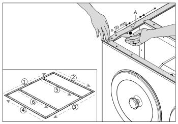
Fig. 4.11 Removal of backing material
