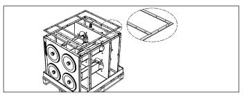
Fig. 4.10 Seals on filter module
