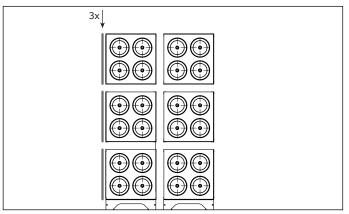
Fig. 4.8 Additional seals on # filter modules
