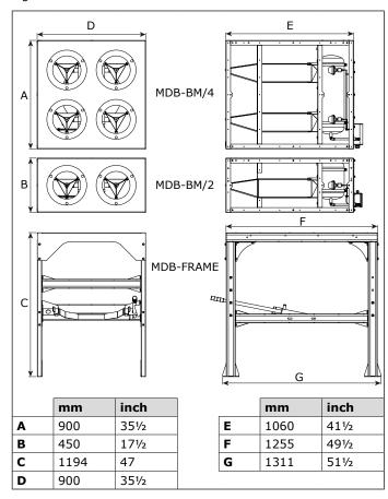
Fig. II Scope of supply
