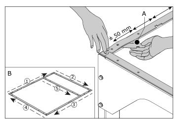
Fig. 4.7 Removal of backing material
