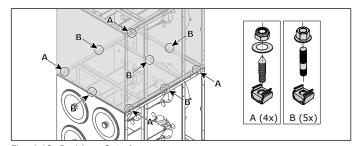
Fig. 4.19 Position of studs
