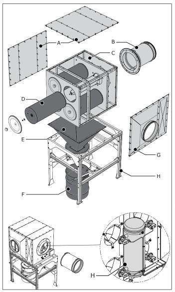
Fig. 2.1 Main components and elements
