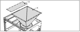
Fig. 4.2 Hopper + cover plate
