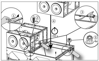
Fig. 4.16 Filter module on second frame
