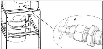
Fig. 6.1 Drain valve
