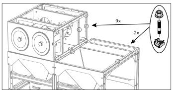
Fig. 4.17 Position of studs
