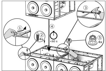
Fig. 4.18 Filter module on first filter module
