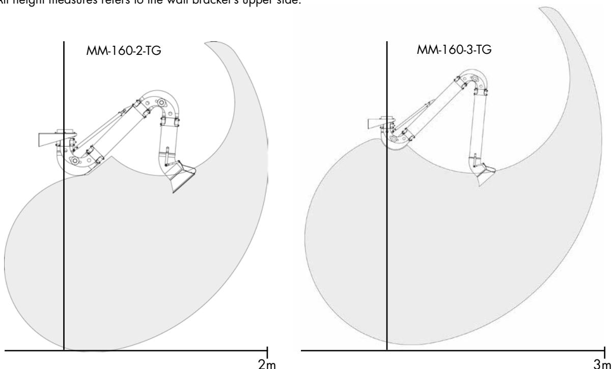
The operating range from a top view. The wall bracket is to be placed in such a way that the place of work is within the shaded area.
