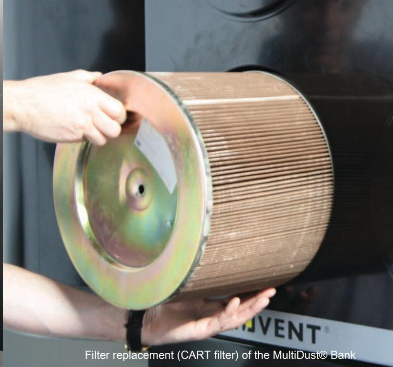
Filter replacement (CART filter) of the MultiDust® Bank
